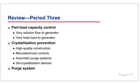
Period Three explained the part-load operation of the absorption chiller. It described the use of energy valves, burner controls, throttling and bypass valves, and adjustable-frequency drives as methods for controlling the capacity on the chiller. Valves and AFDs are used to vary the flow rate of solution to the generator. Modulating energy valves and burner controls are used to vary the heat input to the generator.
